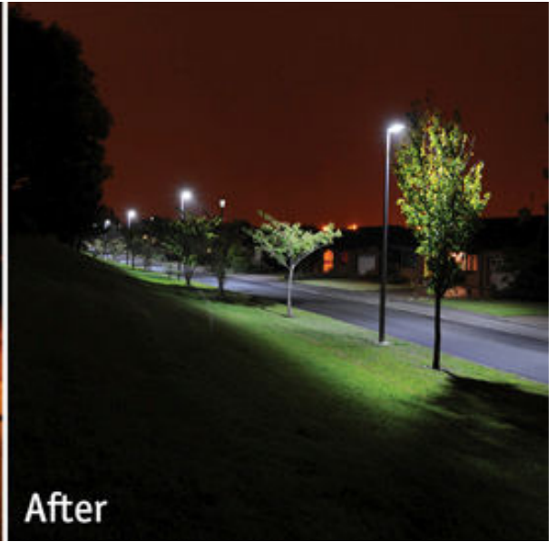
3/18 Pictures of a trial in Middlesbrough showing Before with SOX Lighting and After with LED's.
